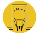
Wheelbarrow equipped with deep and narrow tray, allow easy access through narrow doorway.
